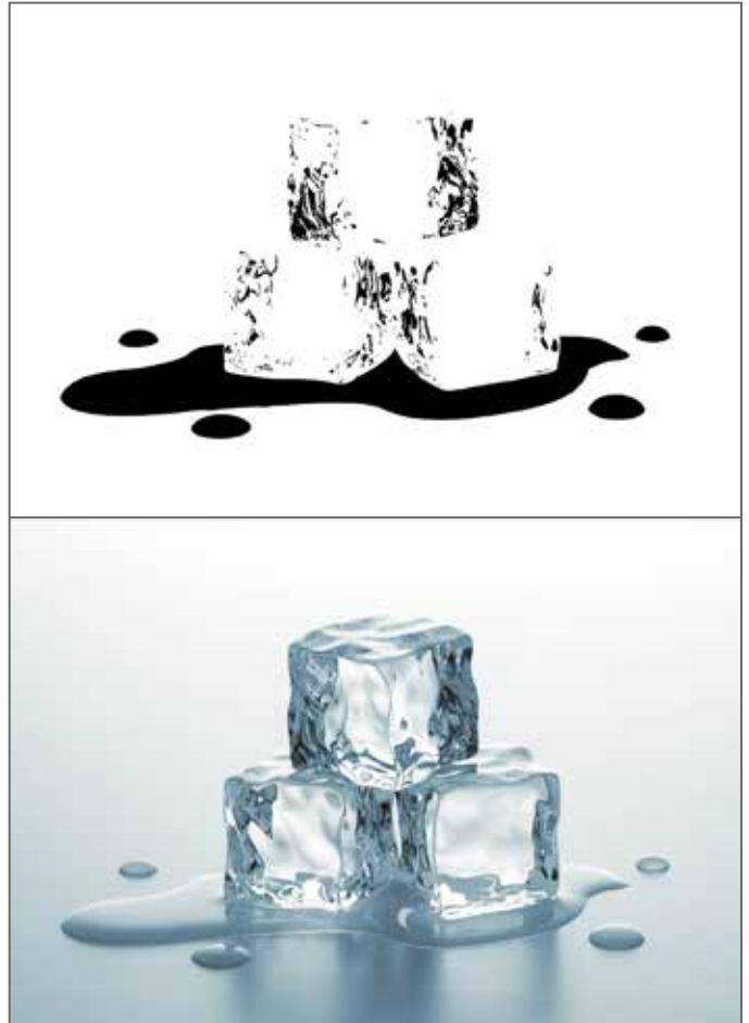
The top image shows the separation of the specific area where spot coating will be applied to the bottom image.
